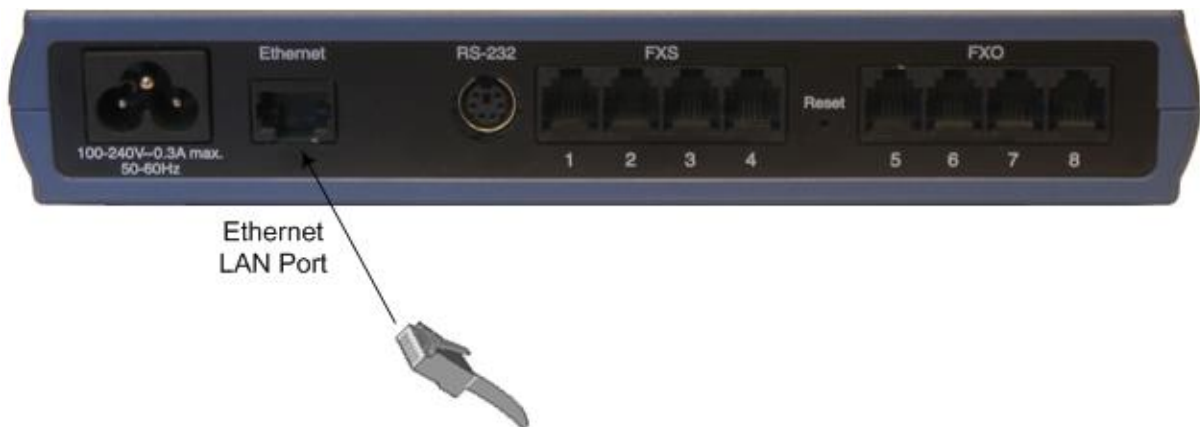
Figure 5-3: Connecting to the Ethernet
