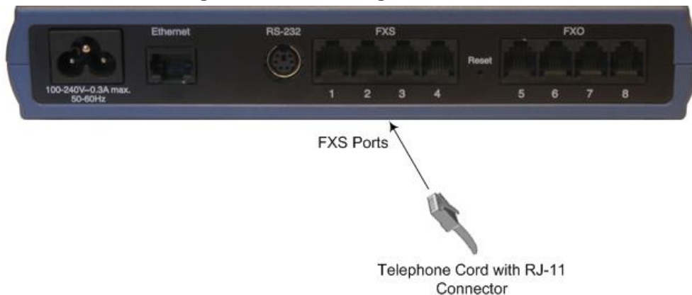
Figure 5-5: Connecting FXS Interfaces
