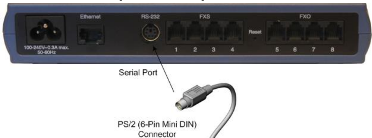
Figure 5-13: Connecting the Serial Port
