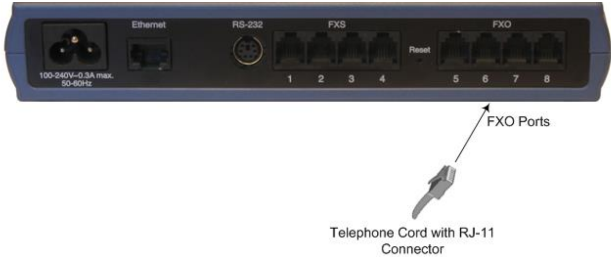
Figure 5-7: Connecting FXO Interfaces
