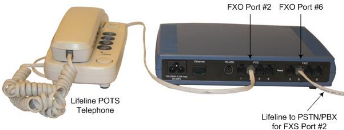
Figure 5-10: Lifeline Cabling for FXS and FXO Devices
