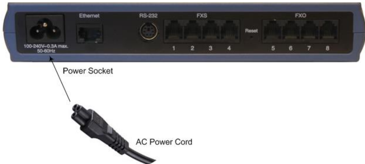
Figure 5-14: Connecting to the Power Supply
