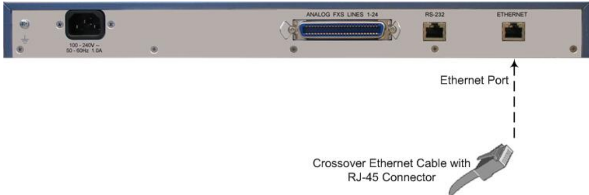
Figure 2-2: MP-124 Ethernet Connection to PC for Initial Connectivity (e.g., MP-124 Rev. E)
